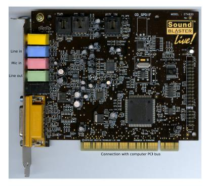
Figure 3.3.: A typical sound card.
